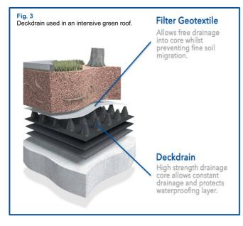
The filter geotextile in Deckdrain is manufactured from up to 95% recycled material making it an environmentally sound choice. Deckdrain comes in rolls of 1.1m x 50m (55sqm/roll) and is easily rolled out and installed. It is flexible which allows it to be bent up against parapet walls, upstand beams, other protrusions and planter boxes.
